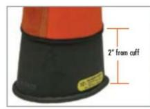
The minimum distance from the leather protector cuff to the bead of the rubber glove for this Class 2 glove is 2 inches.
