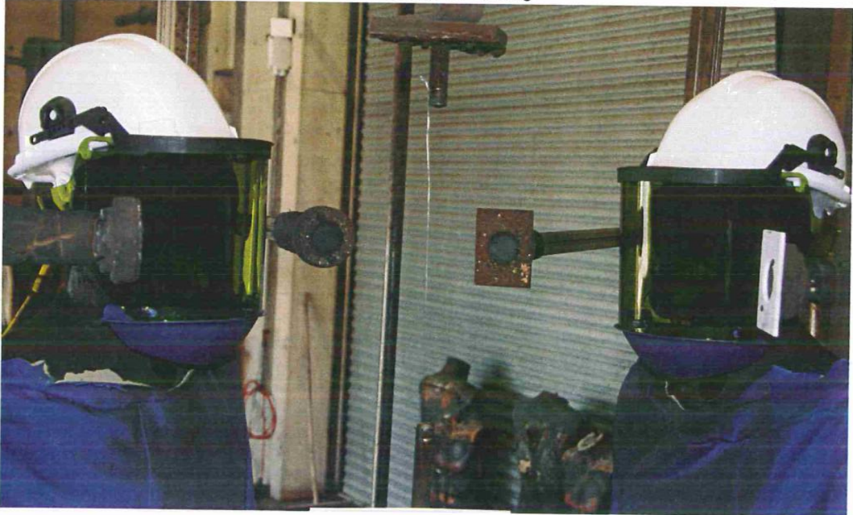
Figure 2: Elvex Faceshield FS-20ARC-10 with Blue chin protector and ProGuard SC30-R6 safety helmet As set up for testing
