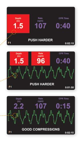
The ZOLL AED 3 BLS can be easily configured to show the CPR Dashboard<sup>™</sup> only, or both the CPR Dashboard and ECG. Depth and rate indicators are highlighted in red if the compression rate is too slow and/or the depth is too shallow when in adult rescue mode.
