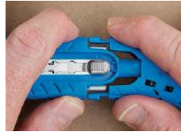
Squeeze release tabs and pull the handles apart
