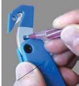
FILM CUTTER CHANGE Use ball point pen (above) to remove & replace film cutter unit.
