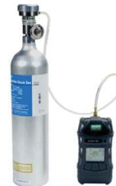
Manual Testing with Test Gas
